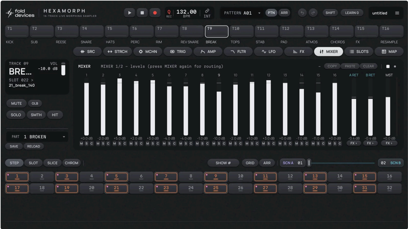
THE MIXER: 16 TRACKS, TWO BUSES AND THE MASTER
